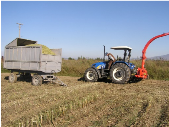
Figure 2. The two row PTFH switching trailer
