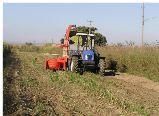
Figure 4. The two row PTFH working with system A
