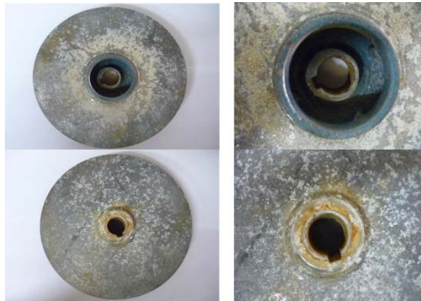
Figure 3. The wear on the impeller after 180 hours of operation (Yüksel & Eker, 2010).
