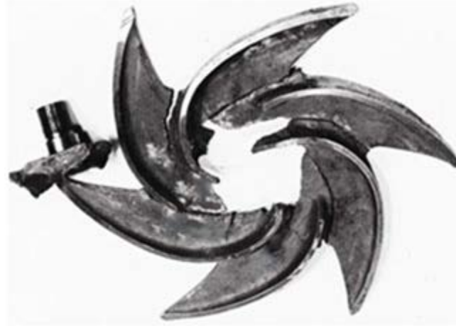
Figure 11. Stressed corrosion centrifugal pump impeller (Cebeci, 2016).
