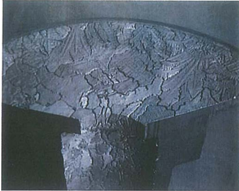
Figure 6. Centrifugal pump seal bed with intergranular corrosion (Cebeci, 2016).
