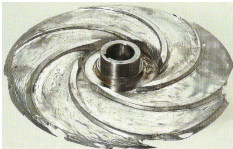
Figure 5. Waveform erosion-corroded impeller (Oluk & Ozturk, 2011).
