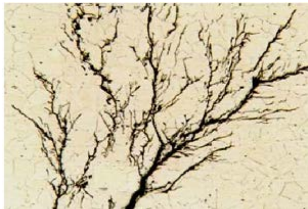
Figure 10. Wear as a result of fatigue (Zeren, 2017).
