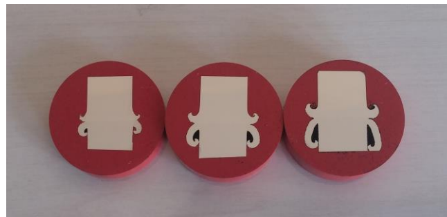
Fig. 3. Macro-photograph of welded and polished samples.
