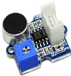
Figure 1. Grove sound sensor and cable connection table
