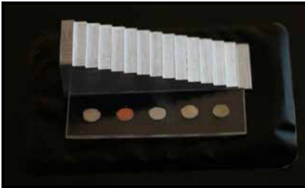
Figure 1: Storage phosphor plate with root-canal filling material samples and aluminum stepwedge in place for radiographic exposure.
