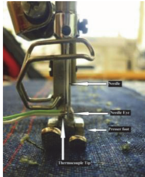
Figure 7. Needle temperature measured by the thermocouple touch method (6)
